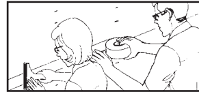
4. ...and tape seams with pressure sensitive aluminum tape.
